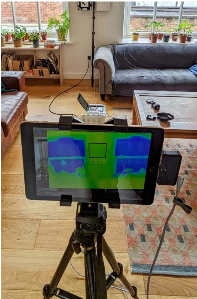
Left: In-situ U-value testing.
