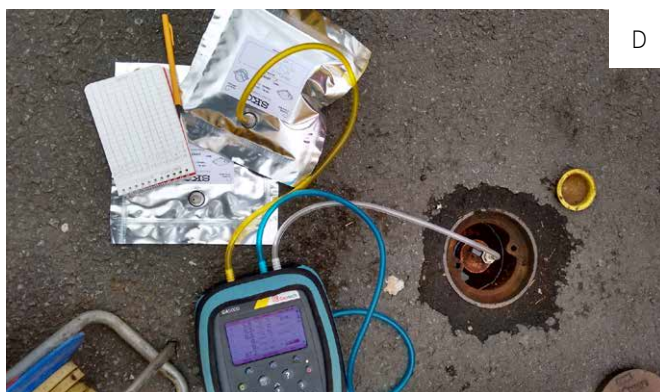
A. Cross-section showing Nantwich deposit sequence. © Caroline Malim B. Drilling in 2007 using a windowless sampler rig, steel casing and Perspex tubes. © Tim Malim C. Recording extracted core in a Perspex tube. © Tim Malim D. Gas sampling from one of the dipwells, using a GA 5000 analyser and Tedlar bags for the C14 gas sample. © Tim Malim
