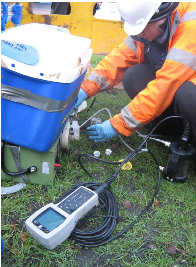
Water sampling using a low-flow cell with a multi-probe water quality meter and a peristaltic pump. © Tim Malim
