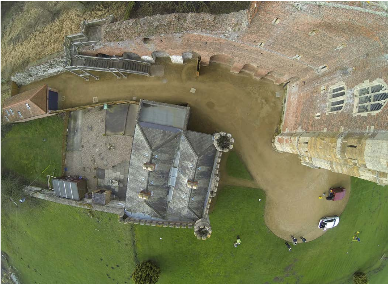
Figure 21 Severe image distortion from a recreational camera. © Skyline images
