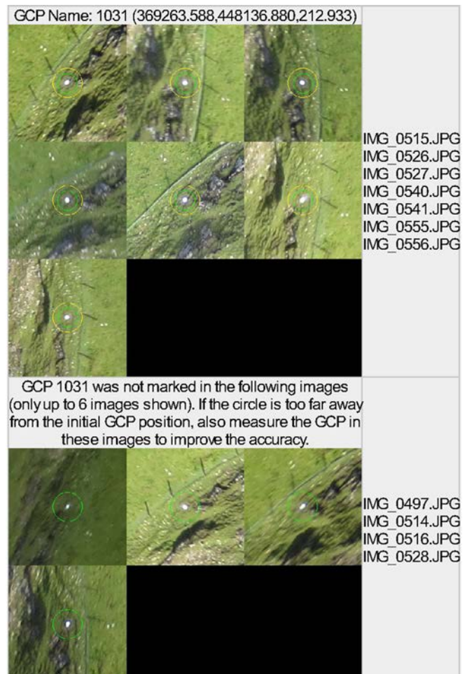
Figure 70 Poor images taken from a fixed-wing SUA under windy conditions: GCPs shown.
