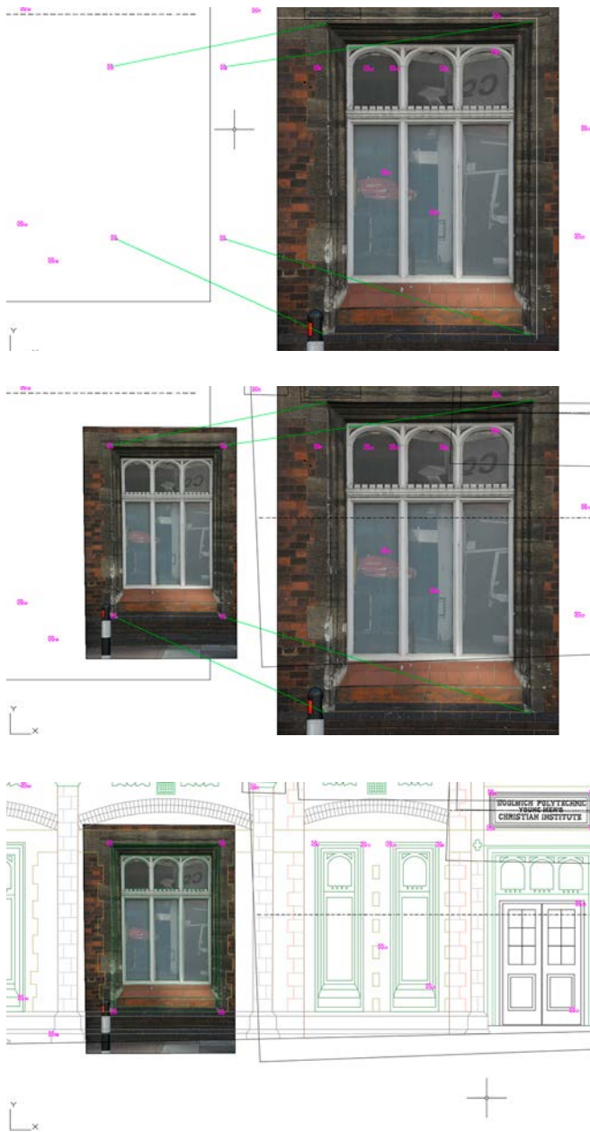
Figure 10 Stages of single image rectification.
