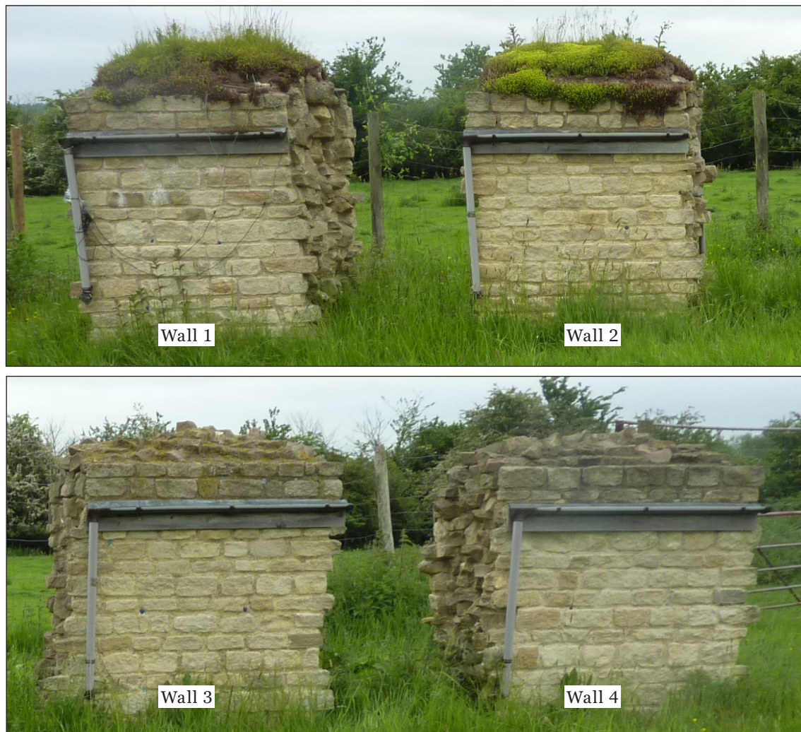
Figure 4.26 Lichen colonisation on the Wytham Woods test walls.
