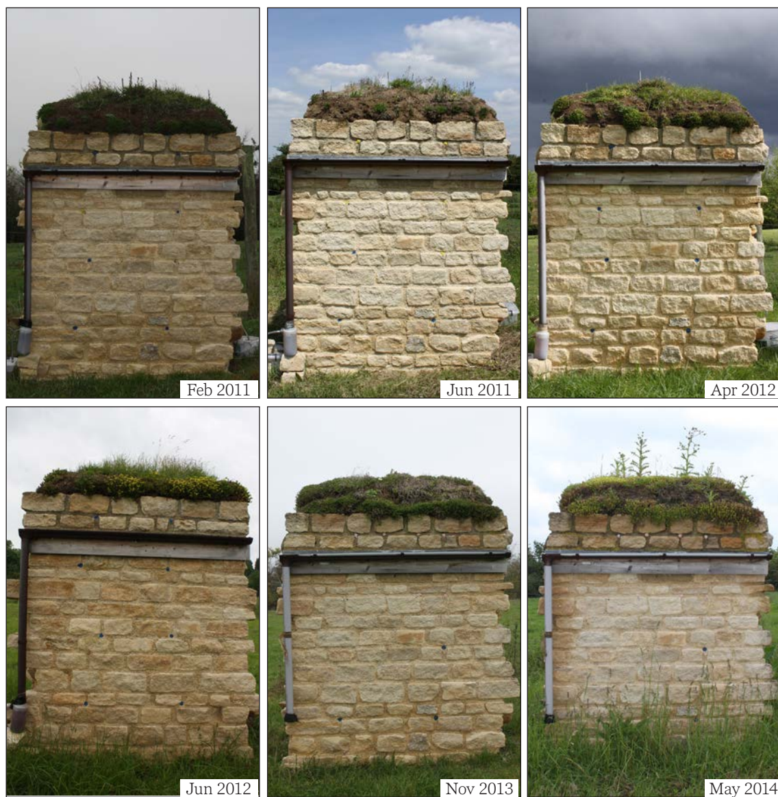
Figure 4.34 Changing appearance of soft capping on the Wytham Woods test walls. ©Heather Viles, University of Oxford
