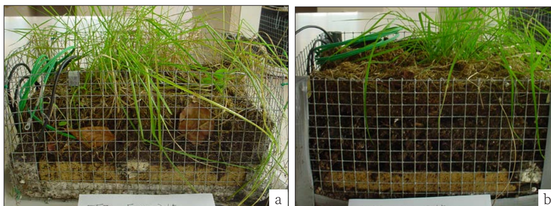
Figure 3.2 (a) 5-cm and (b) 10-cm thick soft caps after the ‘Long term field experiment’. ©Heather Viles, University of Oxford
