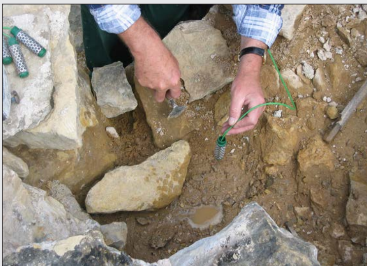
Figure 3.8 Emplacement of the Watermark sensor in the hard capping at Byland Abbey. © Chris Wood, Historic England
